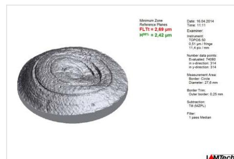
The Relief image provides an additional visual impression about the form of the surface of the part.
