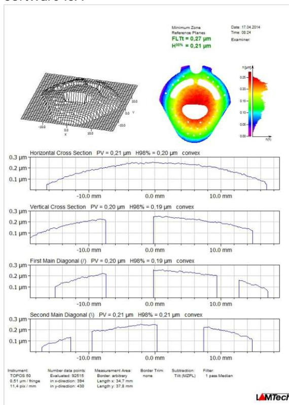
The Measurement Sheet summarizes the measurement results for a simplified documentation.
