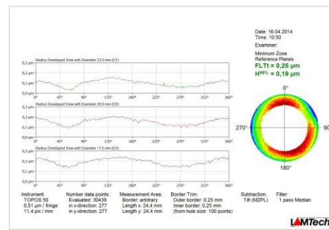
The Radius Developed Views provide the possibility to evaluate the part at any diameter.
