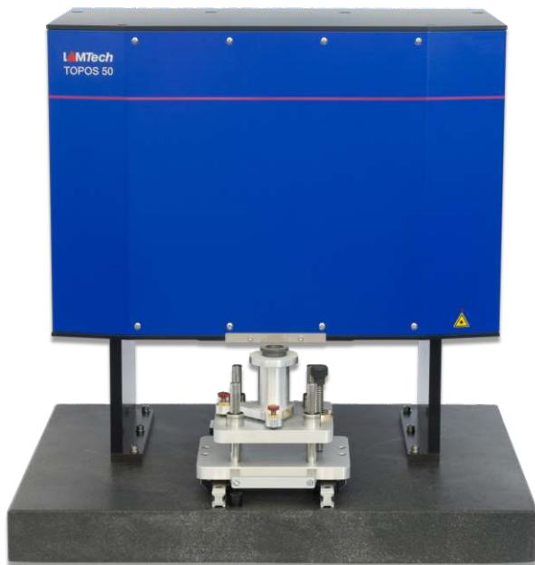
The TOPOS 50 is a non-contact flatness measurement instrument for precision-manufactured surfaces with sub-micron accuracy. Based on the well-proven TOPOS 50, the new version now also offers a motor-driven adjusting mechanism of the sensitivity setting, like it is already known from the TOPOS 100. Thanks to the new design, the TOPOS 50 now optically blends in with the TOPOS series.
